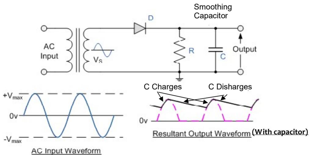
**Fig.2: Half-wave rectifier circuit with capacitor filter**
